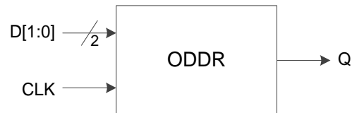
Figure 3-15 I/O Logic in DDR Output Mode
