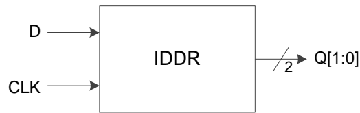
Figure 3-14 I/O Logic in DDR Input Mode
