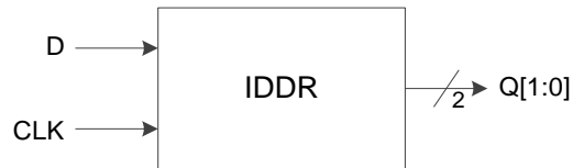
Figure 3-15 I/O Logic in DDR Input Mode
