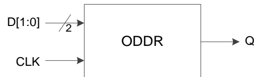
Figure 3-16 I/O Logic in DDR Output Mode
