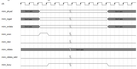
Figure4-31 The Write Timing of miim
