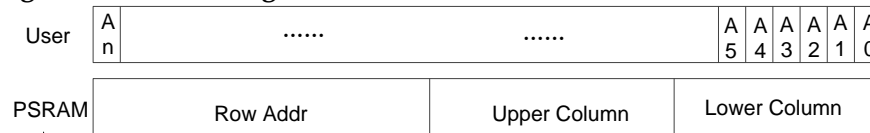
Figure 4-5 Addressing Scheme in Row-Column Order
