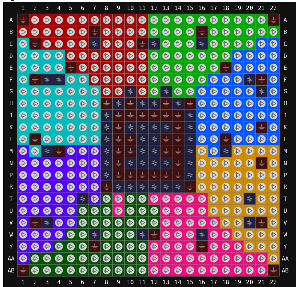
Figure 3-11 GW2A-18 UG484 View of Pins Distribution
