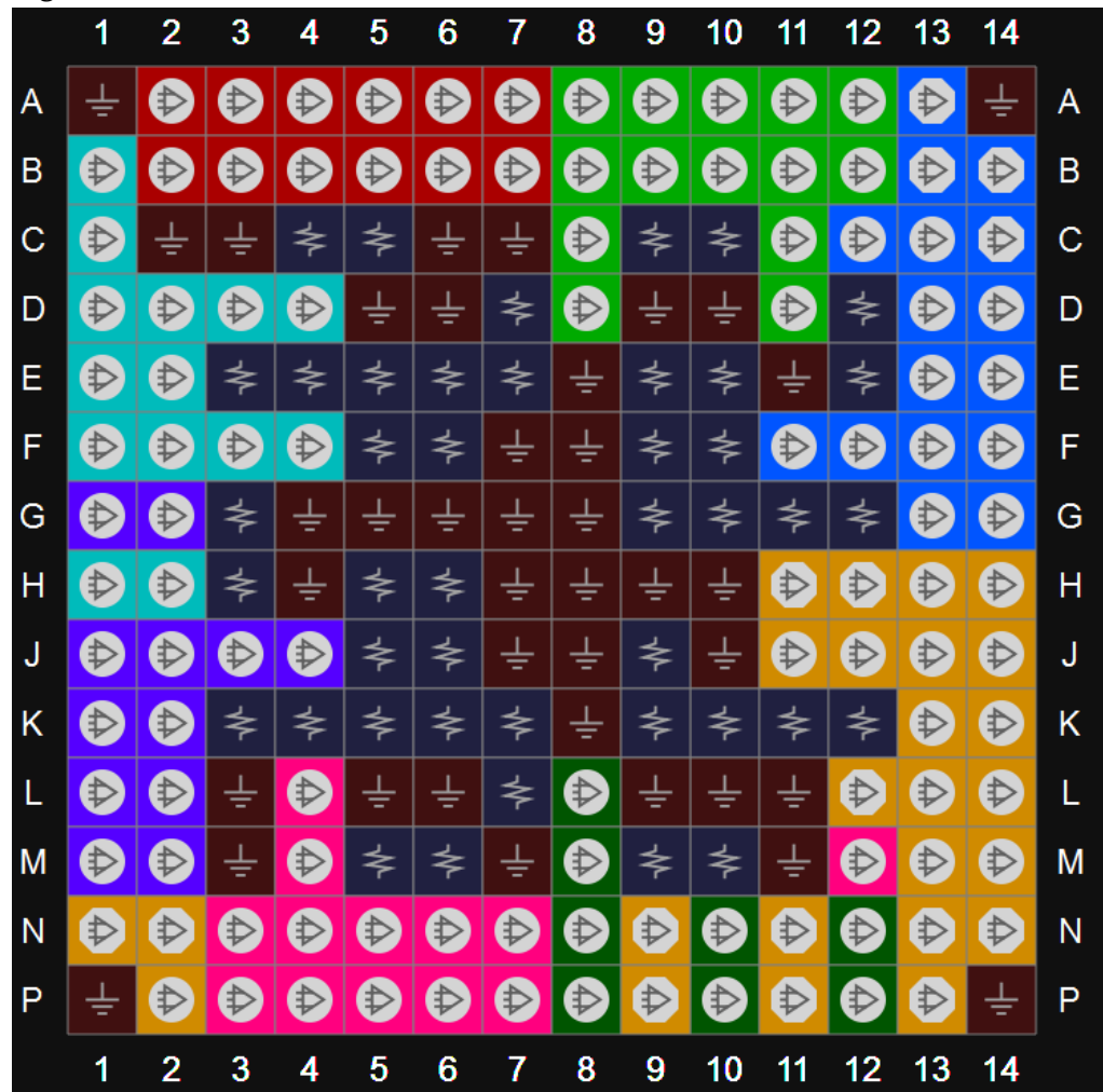
Figure 3-3 GW2A-18 MG196 View of Pins Distribution
