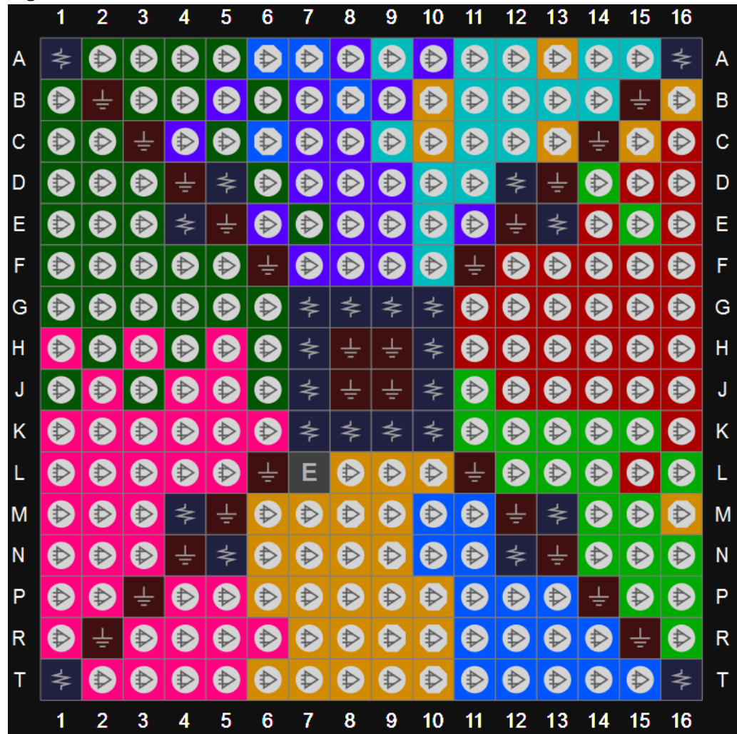
Figure 3-4 GW2A-18 PG256View of Pins Distribution
