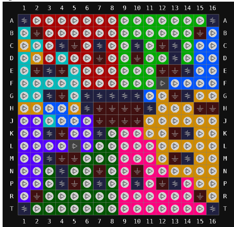
Figure 3-12 GW2A-18 PG256CF View of Pins Distribution
