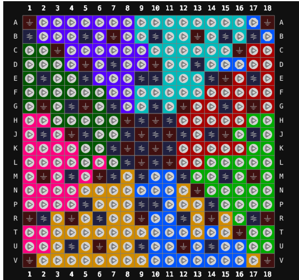
Figure 3-14 View of GW2A-55 UG324 Pin Distribution
