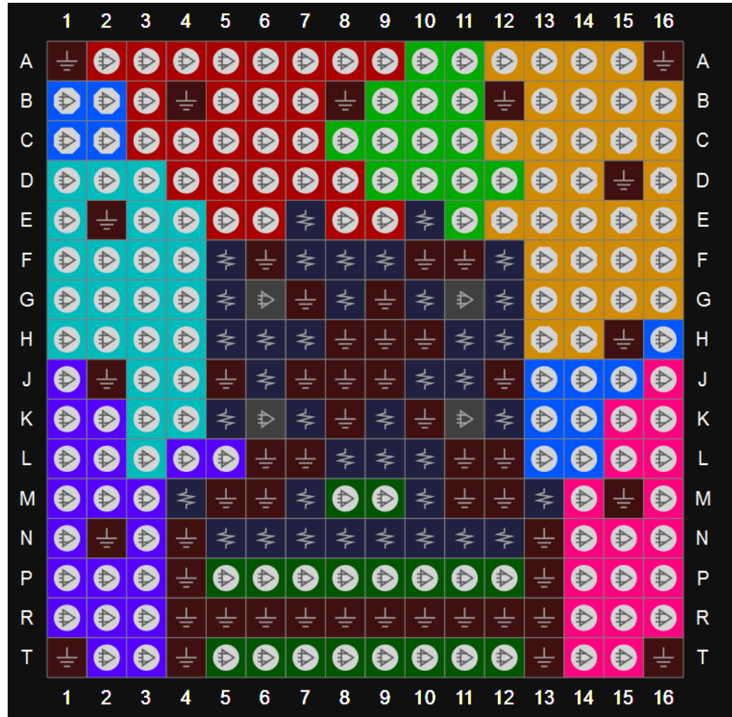
Figure 3-10 GW2A-18 PG256E View of Pins Distribution
