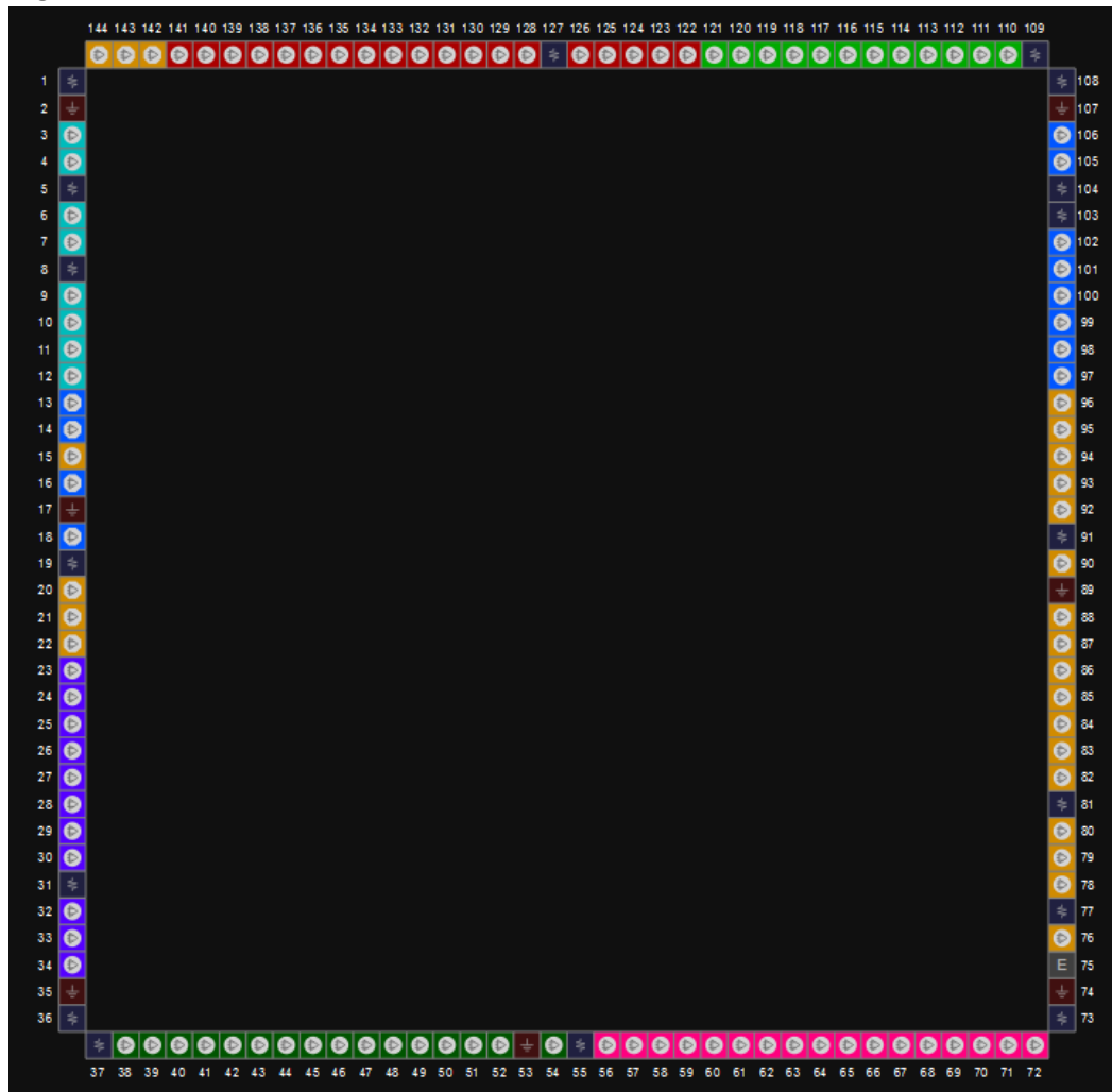
Figure 3-2 GW2A-18 EQ144 View of Pins Distribution
