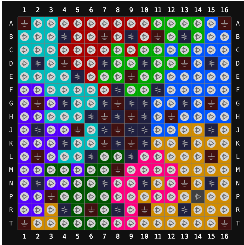
Figure 3-13 GW2A-18 PG256SF View of Pins Distribution
