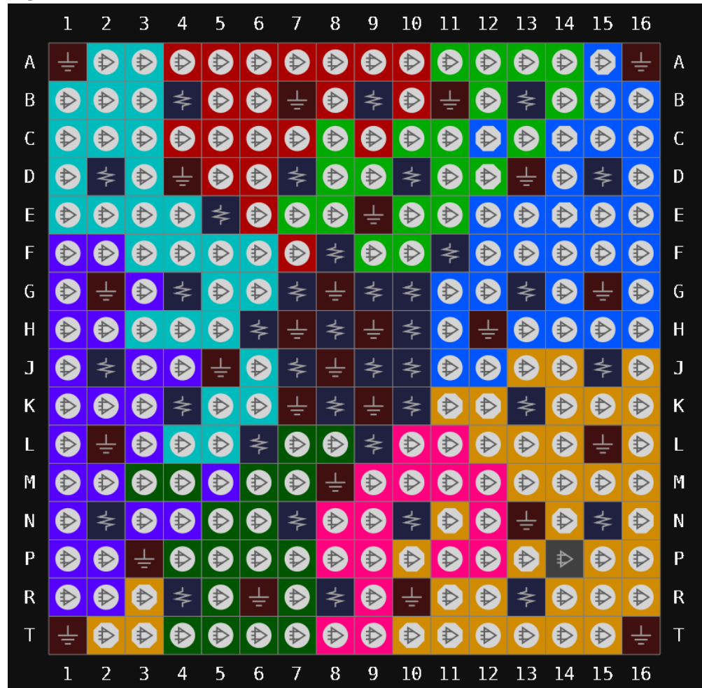
Figure 3-5 GW2A-18 PG256S View of Pins Distribution
