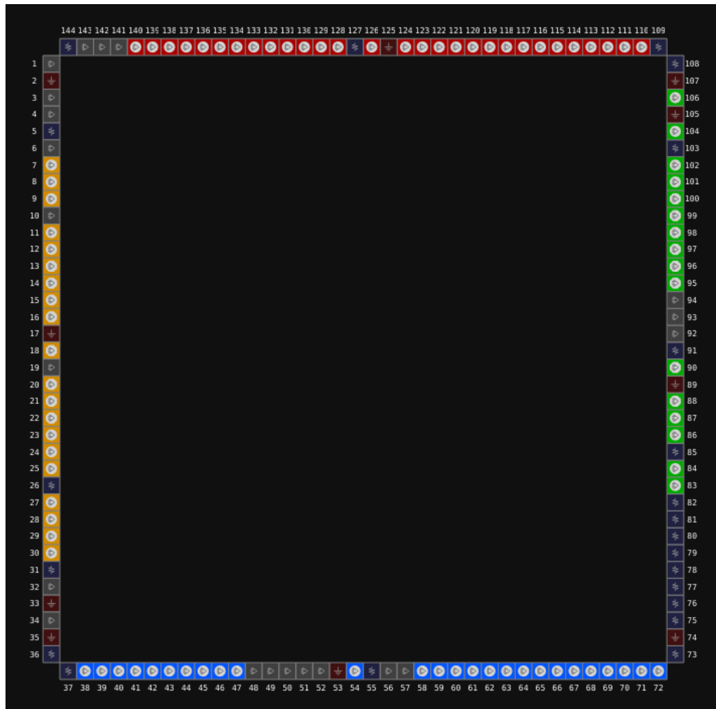
Figure 3-2 View of GW1NSE-2C LQ144 Pins Distribution (Top View)
