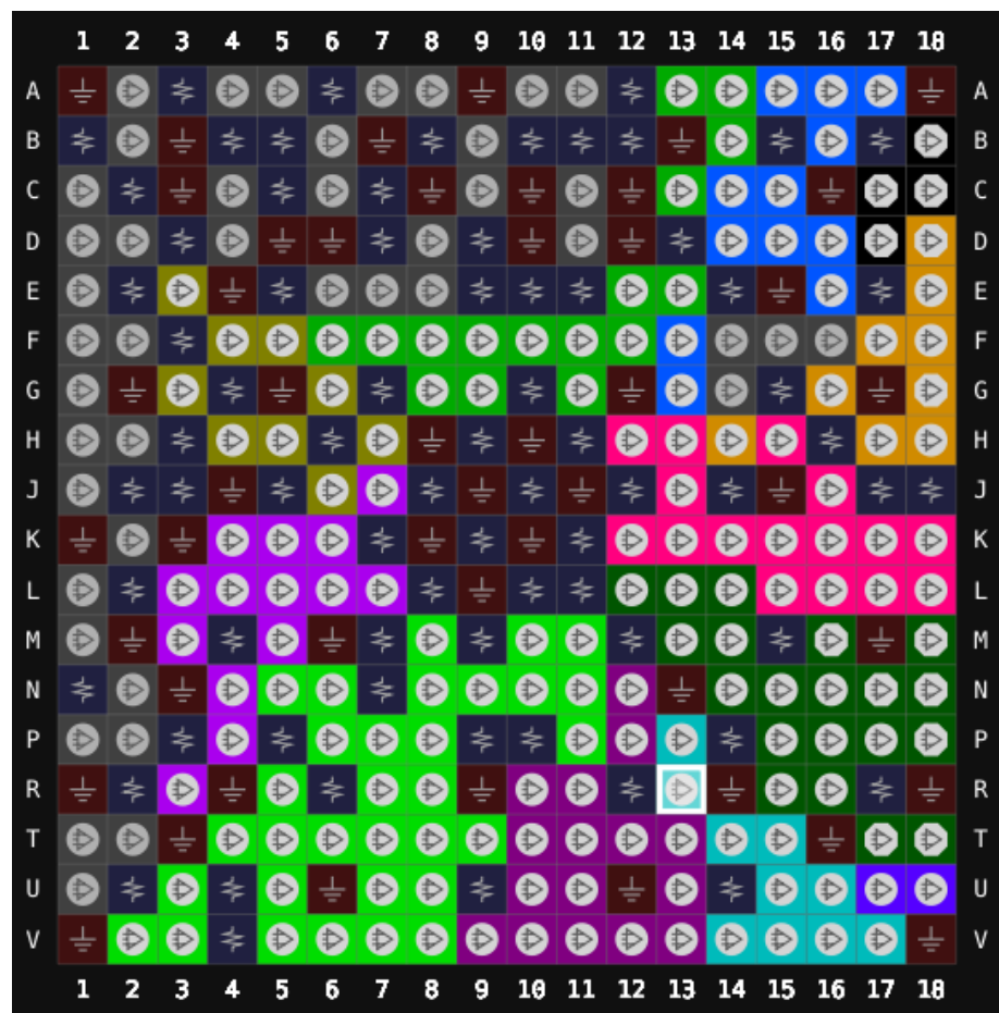
Figure 3-8 View of GW5AT-60 UG324 Pin Distribution (Top View)
