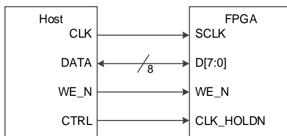
Figure 5-29 Connection Diagram for CPU Mode
